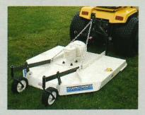
The optional Bush Hog rotary cut mower gives you high-speed cutting capability for mowing through large fields. It features a wide cutting width of 42" and can be adjusted from 1" to 6" cutting heights. Available for models 1572, 1872 or 2072.
