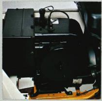
Cub Cadet's 12 H.P. Kohler engine features a solid state inductive electronic ignition which produces a stronger spark for easy, cold-weather starting. Newly designed pistons control oil use, reduce vibration and noise. Balance gears minimize vibration,
